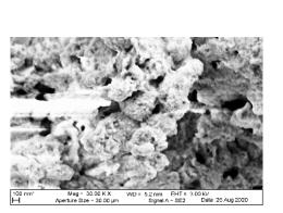
Fig. 3(C) FE-SEM images of the produced CeF<sub>3+x</sub>(①、②)
